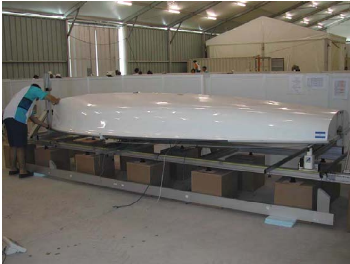
470 Jig with a hull on top (left) and the modular framing and levelling screws detail (right)
