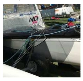
It is clear the **forestay** is affixed on an adjustable plate to the upper briddle, which is therefore the forestay briddle defined in CR F.6.2.(a)(1). Hence, it is as clear that the **tack point** is below the apex of the bridle wire, contravening CR C.10.3 (a)(2).
