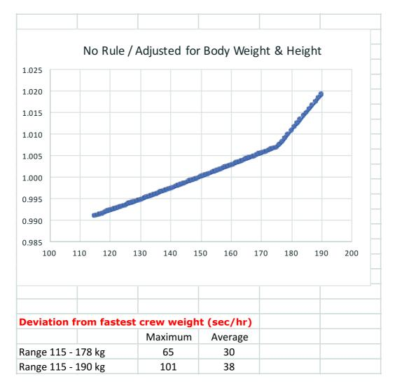
This graph shows the implied handicap rating (Y-axis) for a given crew weight (X-axis) if we would not use any correction for crew weight. The table below the graph provides the maximum and average time differences (expressed in seconds per hour of racing) between the fastest team (115 kg) and the teams within mentioned crew weight ranges (115-178 kg and 115-190 kg).
